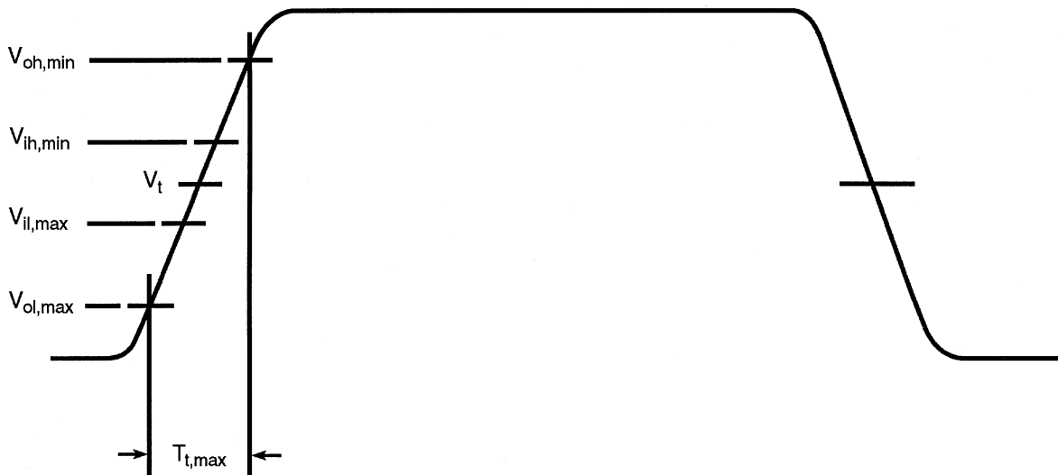
FIGURE C1—VOLTAGE LEVELS AND TRIP POINTS
